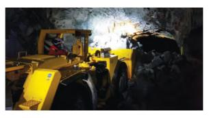
Above: A wheeled loader in an adit during construction of the Cononish mine Below: The processing building is cut into the mountainside
