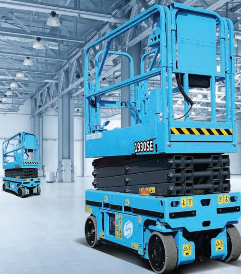
Efficient and environmentally friendly, the Sinoboom electric scissor lift series features platform heights from 4m (12'6") to 14m (45'3") and offers numerous benefits: exclusive open chassis design for reduced daily maintenance time; bumper rail protection; lower cost of ownership and highly versatile parts and components.
