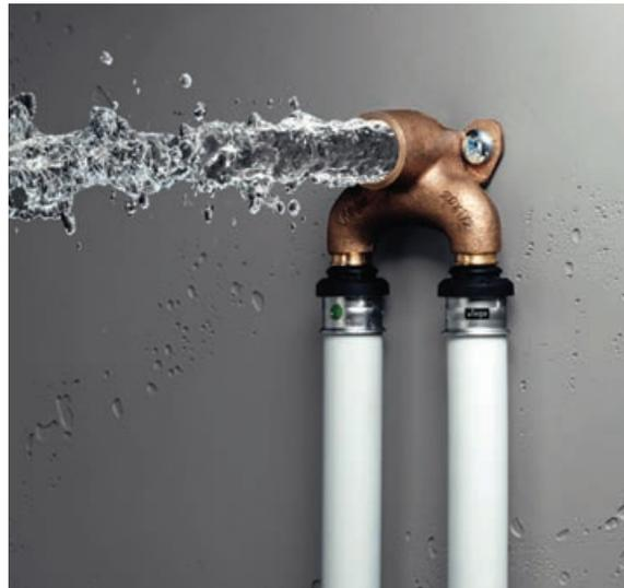
The O-ring is replaced in all Viega Smartpress connectors with a robust and durable polyphenylsulfone (PPSU) support structure which, when pressed, creates a seal across the entire connected surface between the pipe and the fitting. There is no need to widen, deburr or calibrate the pipe, and without an O-ring there is no risk of damaging the seal and causing a leak.
