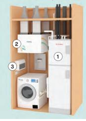
1 Top - Heating and cooling system expansion vessels, valves and connections out to heating, cooling and DHW circuits Mid - Indirect, domestic hot-water cylinder Bottom - Heat pump and heat exchangers
