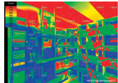
The Daylight Visualizer applies false colour mapping to highlight daylight distribution
