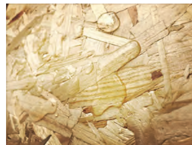
Right: Medite Smartply oriented strand board is moisture resistant
