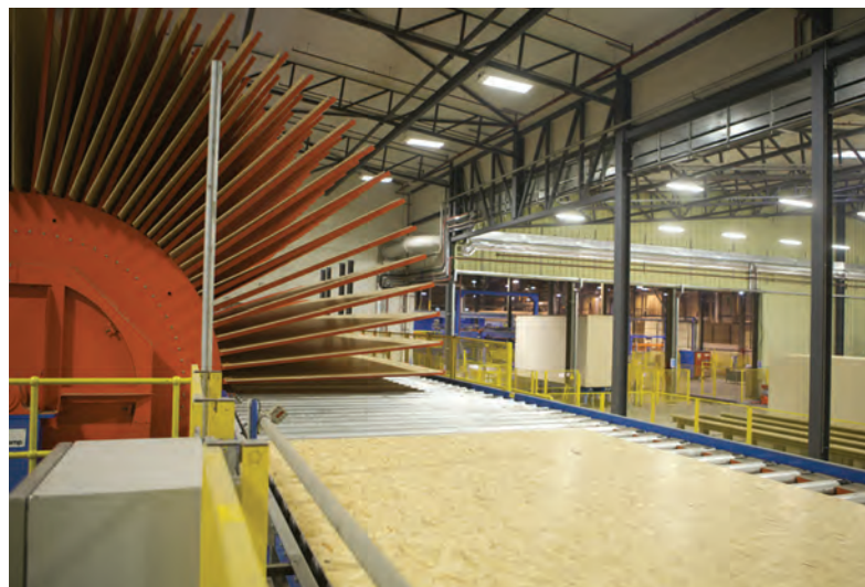
Left: Medite Smartply board drying during the manufacturing process
