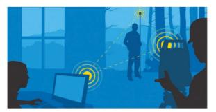
coordinate scan targets, with these then scanned with the laser scanner then identified within a processing software package to register the point cloud. However, with a combined unit such as the GTL-1000, engineers no longer need to set up two different instruments in the same location. Instead, it can all be done in one swift movement, potentially halving the amount of time spent on site.
