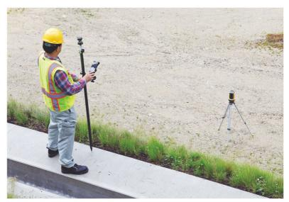
"Construction professionals are able to import and display a digital drawing or a model on the screen of the logger"
